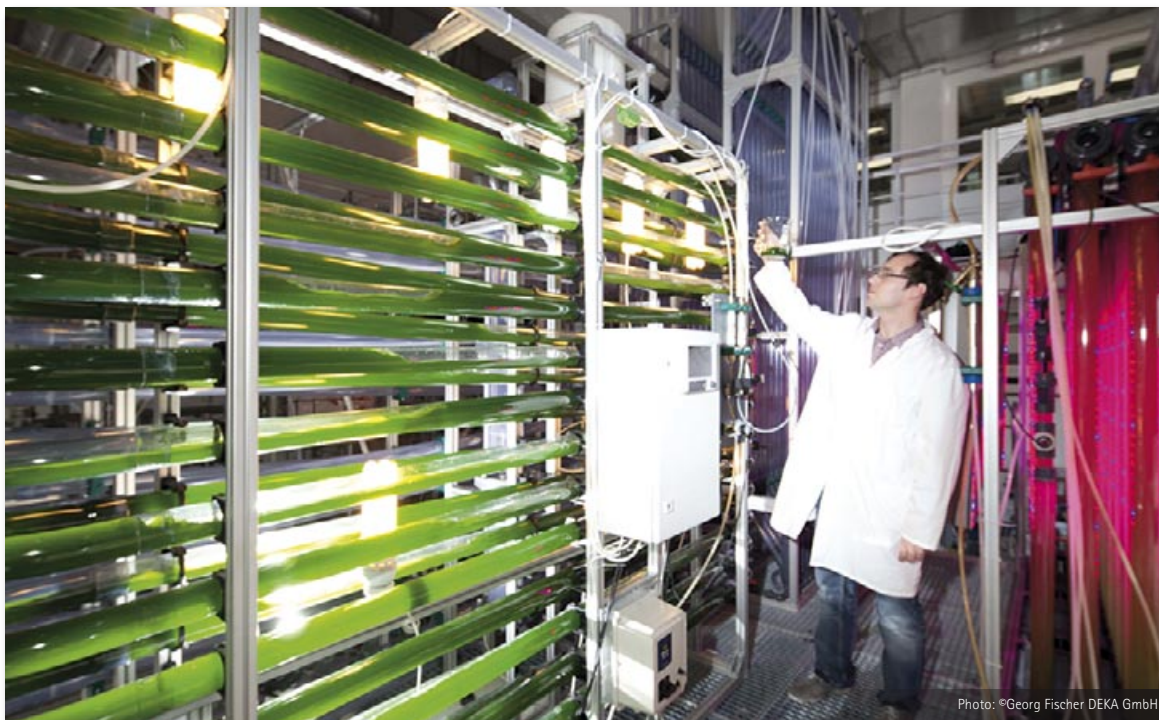
Bioreactors consisting of plastic pipes for the cultivation of algae as a feed material for the cosmetics industry, foodstuffs production and the production of bio-fuels
