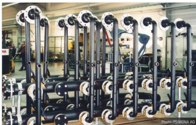
Busbars consisting of electrically conductive polyethylene
