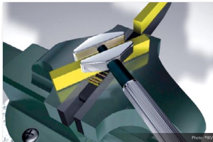
Torsion-shear test for characterisation of mechanical properties of electro-fusion and socket fusion welds
