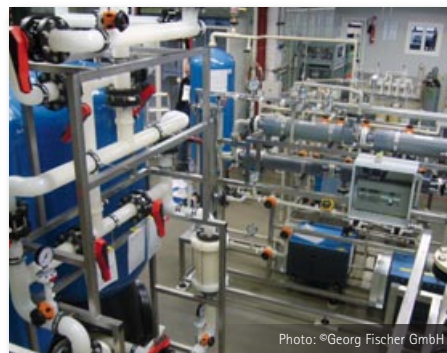
Desalination plant showing PE100 pipes and fittings
